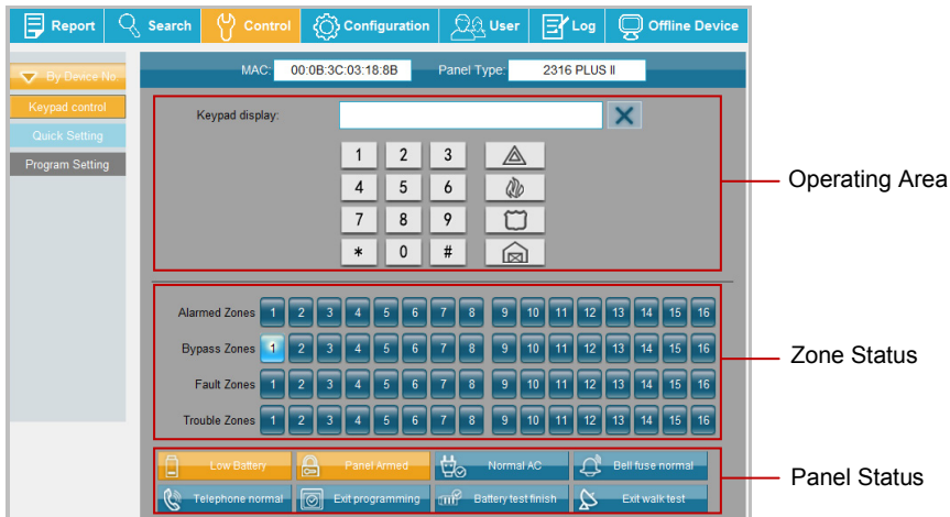
Figure 4-41 Keypad Control (23 Series Panel)
